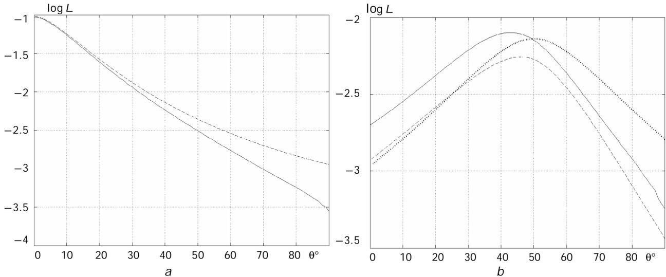
Fig. 1. Brightness body of the light field in a turbid medium ( $\Lambda = 0.8, g = 0.97, \tau = 15$ ): (a)  $\theta_0 = 0^\circ$ , (b)  $\theta_0 = 50^\circ$ .
