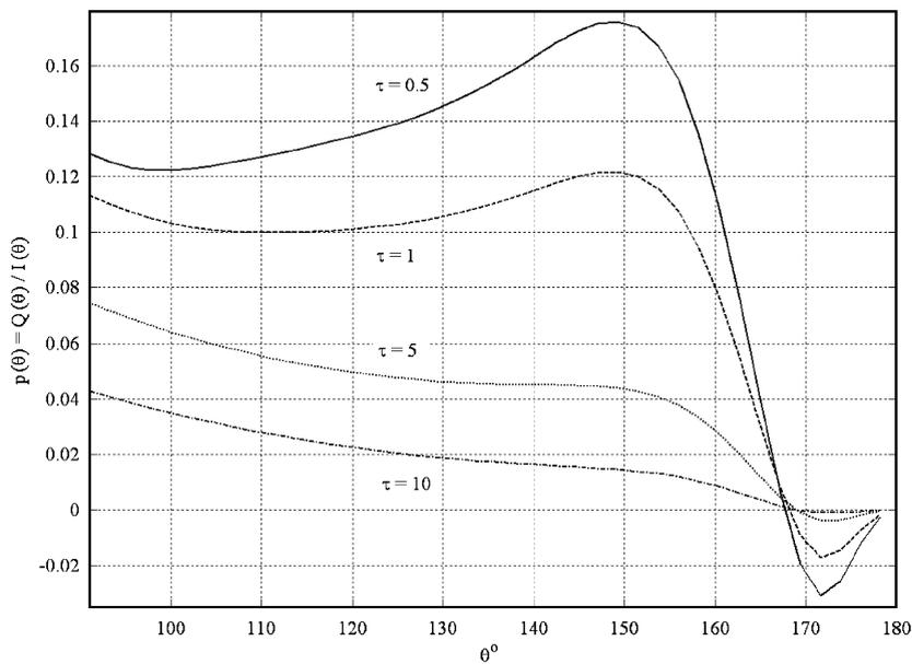
Fig. 16. The spatial dependence of the polarization state  $p(\theta, \tau)$  for Mie-scattering-reflected radiation.
