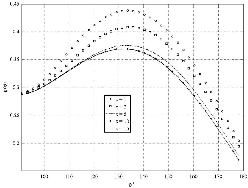
Fig. 19. Spatial dependence  $p(\theta, \tau)$  for reflected radiation and abnormal incident. Henyey–Greenstein scattering matrix parameters are  $g = 0.95$ ,  $P_m = 0.5$ ,  $Q_m = 0.2$ , natural light irradiation angle  $\theta_o = 40^\circ$ , albedo is  $A = 0.8$ .
