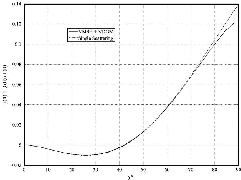
Fig. 11. The polarization degree  $p(\theta)$  dependence for Mie-scattering-transmitted radiation. Slab parameters are  $\tau = 0.1$ ,  $A = 0.9$ . The complete VRTE solution obtained by described VMSH + VDOM method (solid line) is compared with single scattering approximation (dash-dot). Normal irradiation.
