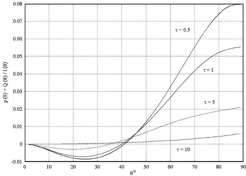
Fig. 15. The spatial dependence of the polarization state  $p(\theta, \tau)$  for Mie-scattering-transmitted radiation.
