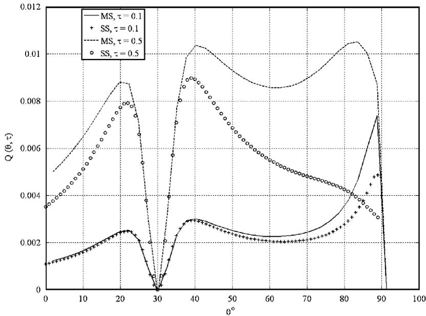
Fig. 17. The spatial dependence of the second component  $Q(\theta, \tau)$  of the Stokes vector for forward hemisphere-transmitted radiation. The irradiation angle is  $\theta_0 = 30^\circ$ , Henyey–Greenstein scattering matrix parameters are  $g = 0.9$ ,  $P_m = 0.5$ ,  $Q_m = 0$ , albedo is  $A = 0.8$ .
