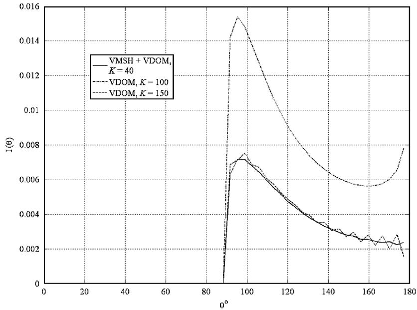
Fig. 13. The efficiency of the proposed method: we compare our method (VMSH + VDOM solid line) with  $K = 40$  expansion terms with standard method of only singularity subtraction—vectorial discrete ordinates method (VDOM—dash-dot and dash lines for different orders of approximation). More long series for standard calculation case are needed. Total intensity is shown.
