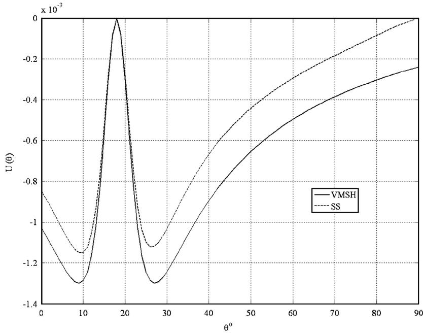
Fig. 9. The third Stokes vector component  $U(\theta)$  zenith dependence for the calculation parameters of Fig. 7.
