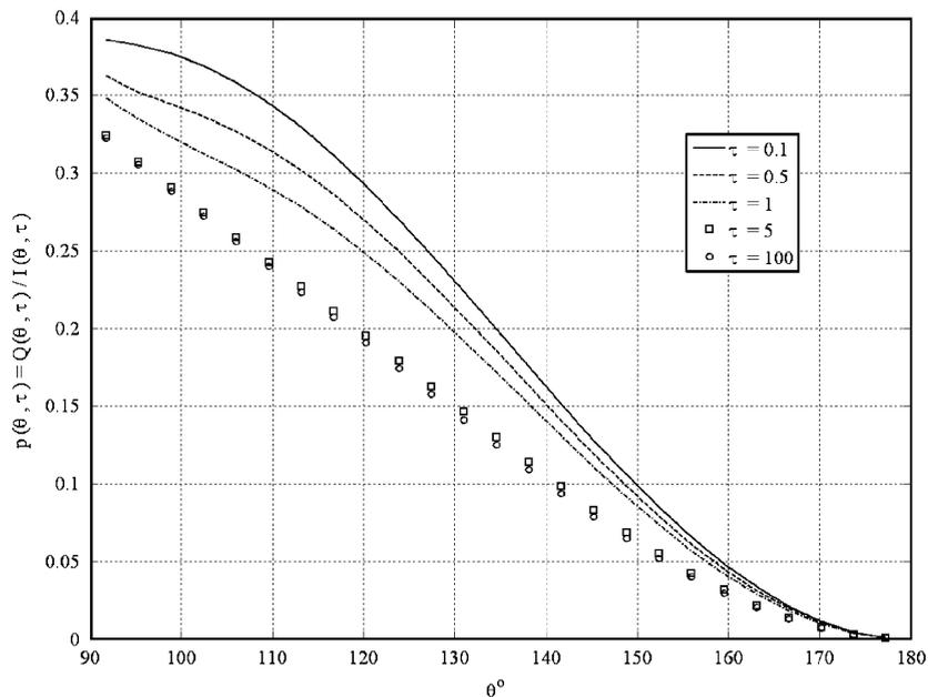
Fig. 14. The spatial dependence of the polarization state  $p(\theta, \tau)$  dependence for Henyey–Greenstein scattering ( $g = 0.9, A = 0.8$ )-reflected radiation.
