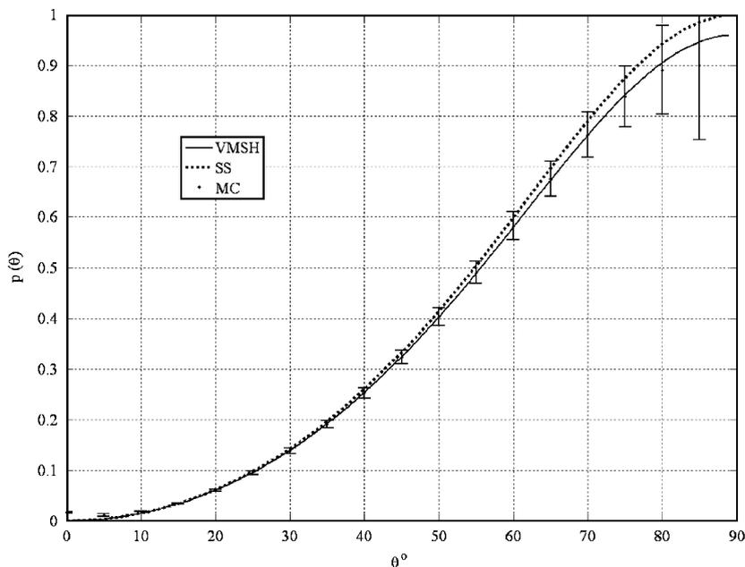
Fig. 4. The polarization degree  $p(\theta)$  dependence for Rayleigh scattering. Slab parameters are  $\tau = 1$ ,  $A = 0.2$ . The VMSH is compared with single scattering approximation (dot) and Monte Carlo simulation (error bar).
